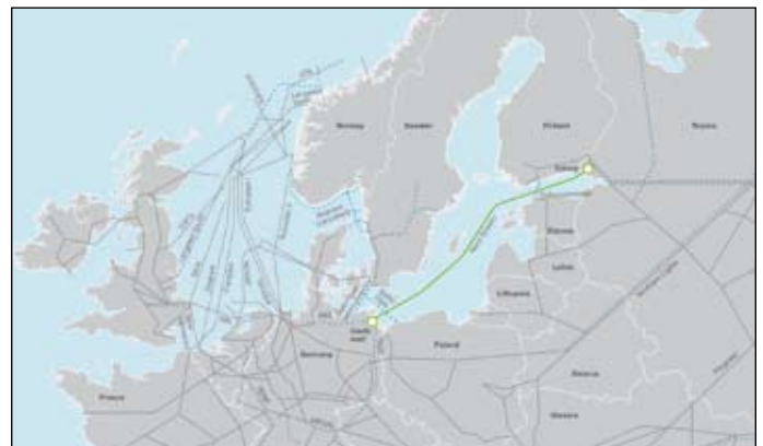
The Nord Stream Project, an offshore natural gas pipeline project due to link Russia and the European Union via the Baltic Sea, will result in two offshore pipelines, each being approximately 1,220 km in length, laid on the seabed of the Baltic Sea.
