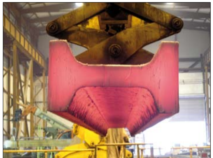
The first beam blanks produced on the X-Cast combination caster for slabs and beam blanks in the works of Peiner Träger, Germany.
