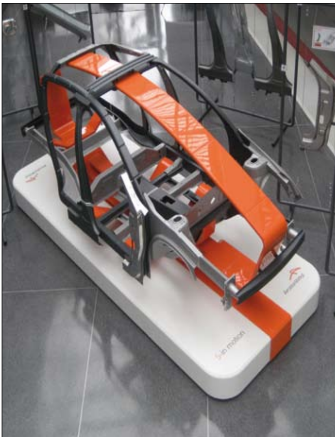
Up to 73kg or 19% of a typical C-segment vehicle's body in white weight can be saved. Photo courtesy of ArcelorMittal
