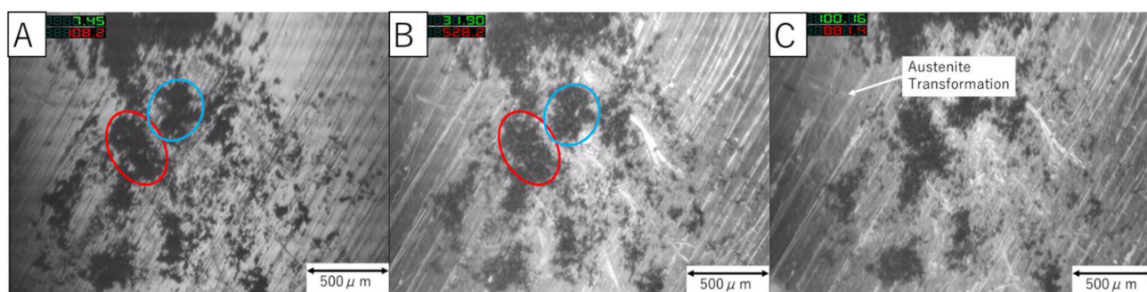
Fig. 10. Laser microscope image of carburization behavior during the heating process in Experiment 2: A,B) Circles of the same color are the same size.
